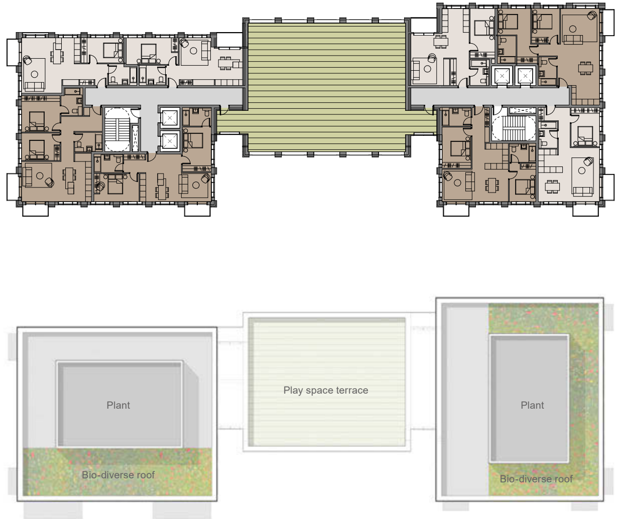
Fig 5.5.31: Roof Plan indicating areas of plant space and bio-diverse roof
